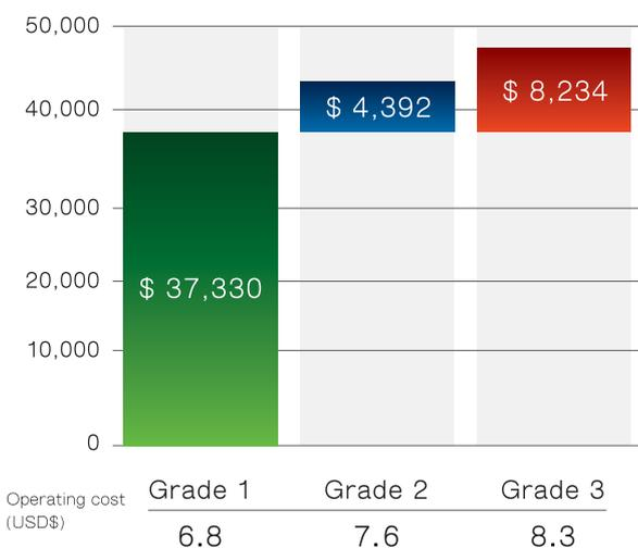
37kW air-cooled air compressor - specific power (kW/m<sup>3</sup>·min<sup>-1</sup>)
